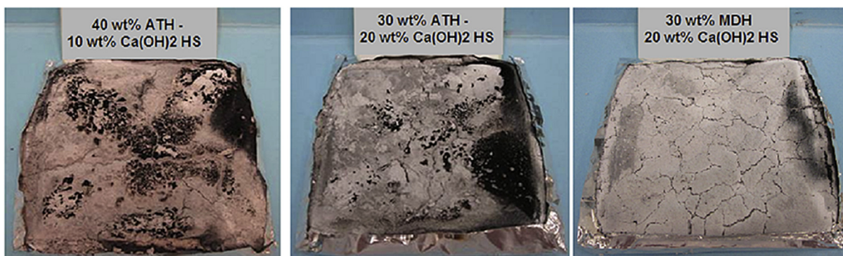
Fig. 9. Pictures of the mass loss combustion residues of MDPE filled with ATH or MDH partially substituted by \text{Ca}(\text{OH})_2\text{HS} .
